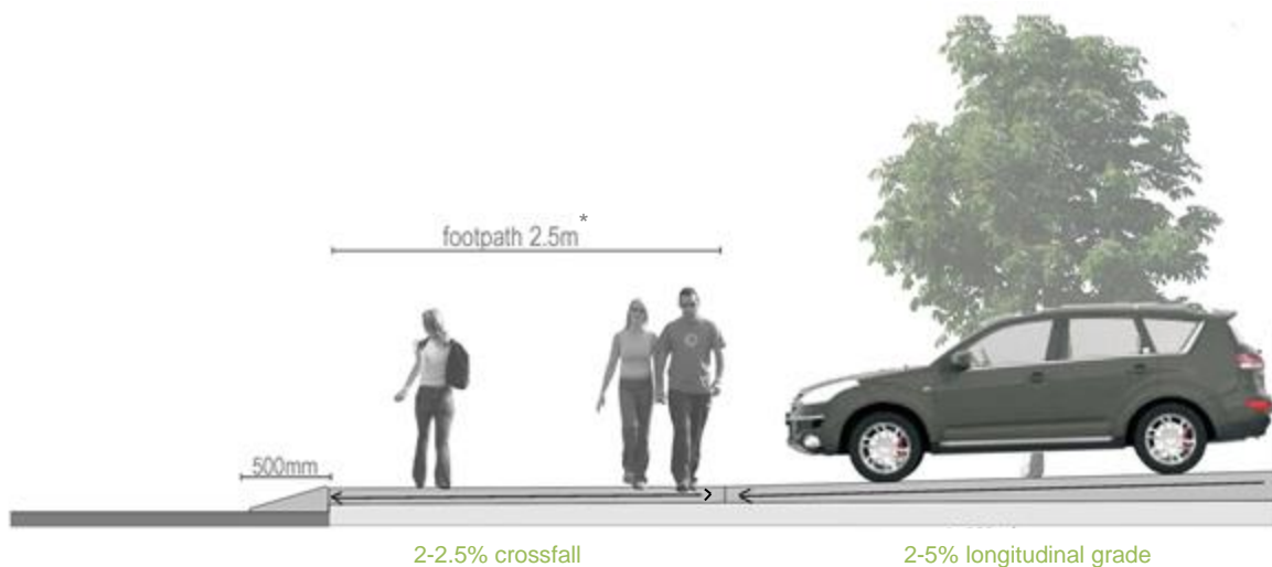
Figure 8 Typical Longitudinal Driveway and Verge Section Design
