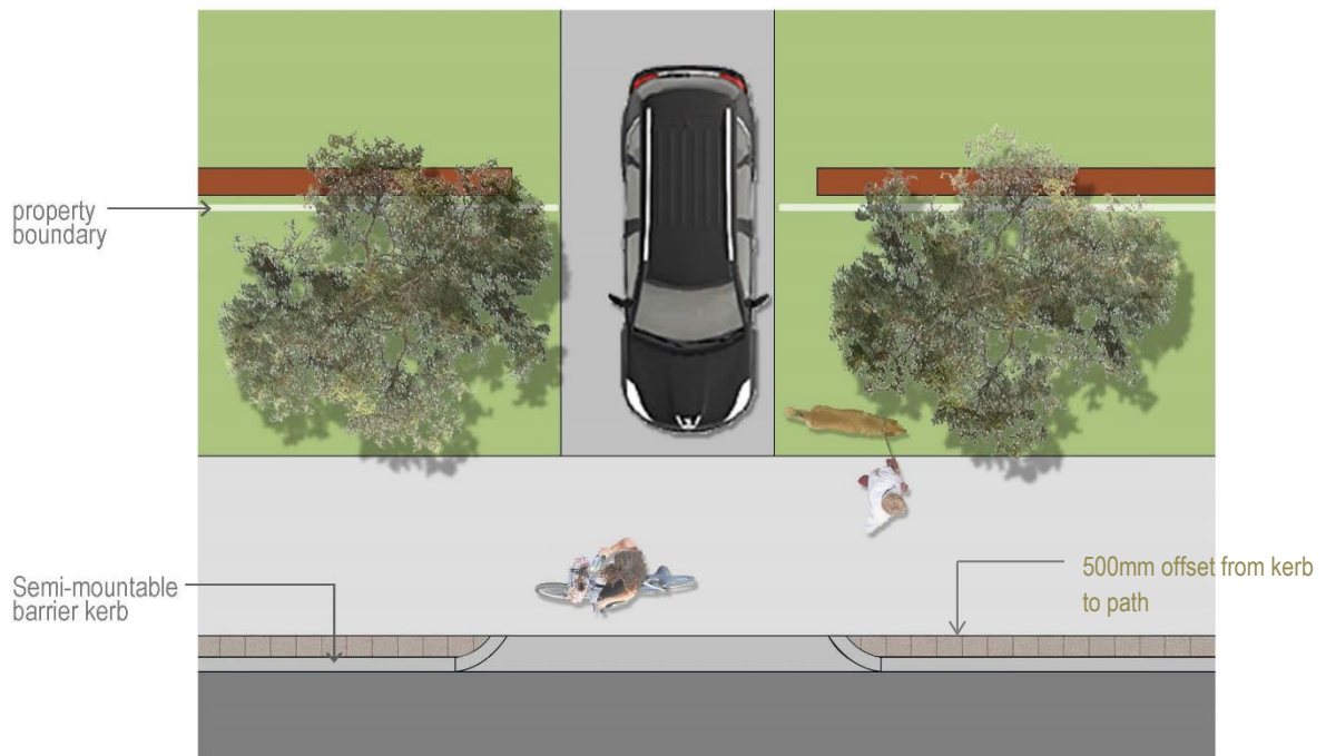
Figure 7 Plan View of Model Crossover Design
