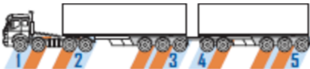
Figure 2.3: Prime mover and semi-trailer towing a dog trailer (pocket road train), length 27.5 m
