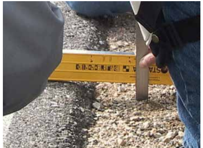
Figure 10.2: Photo of edge drop off height measurement
