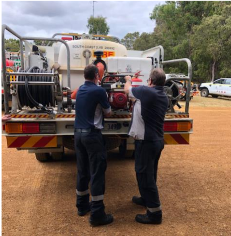
Figure 11: Example of lifting of general equipment (note 2 person lift with above waist height lifting)
