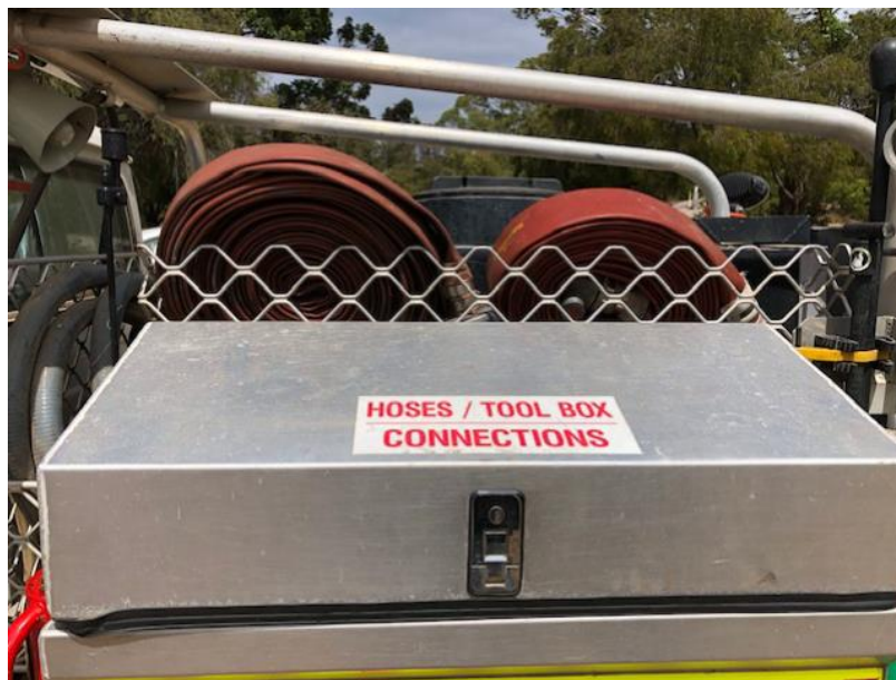
Figure 2: Example of hose reels and tool storage on the back of the vehicles.
